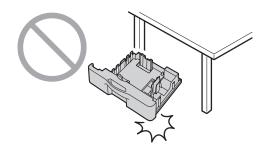
Hold the standard input tray with both hands when removing or installing. The standard input tray weighs approximately 4.8 kg (10.6 lb) when fully loaded with recording paper. Do not touch the plate (9) on the left side of the standard input tray.
